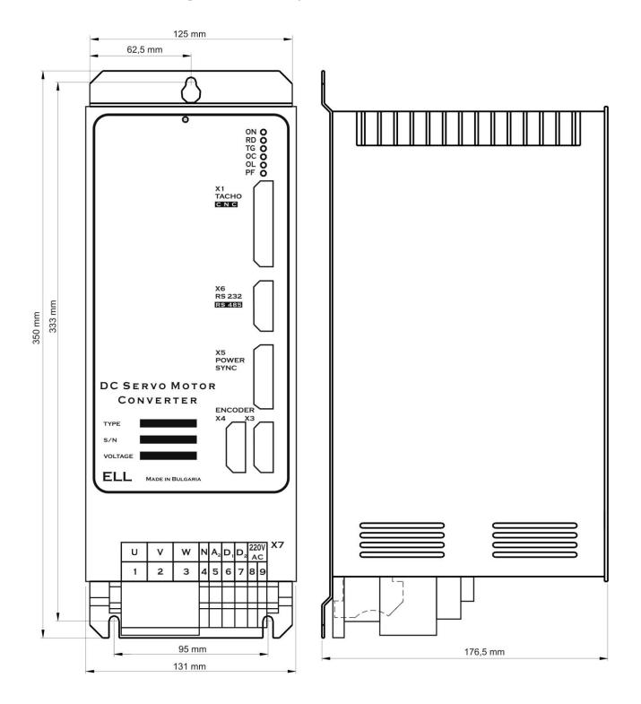
Figure 1 Connecting and overall dimensions of converters type 12030/250 WSM
