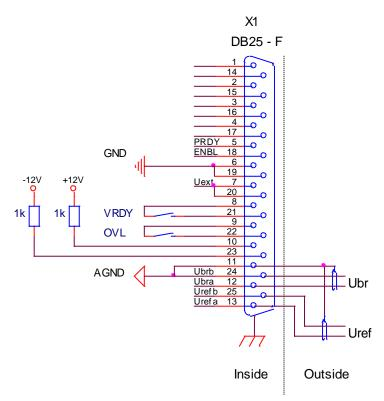
Figure 5 Correspondence of signals and pins of the terminal signal's interface X1
