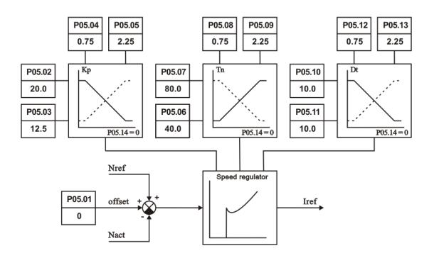
B Speed regulator with adaptation in function of real speed
