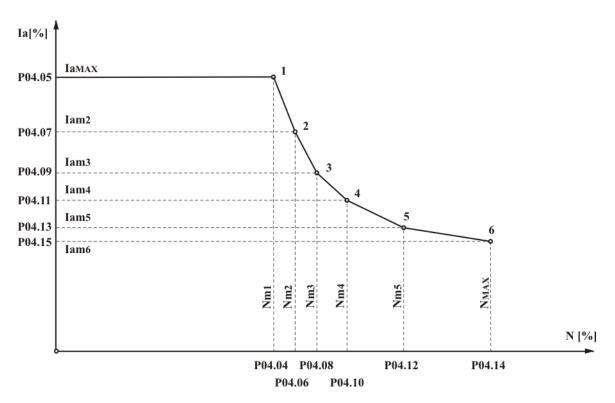
Figure 14 Graphic of dynamic current limit characteristic
