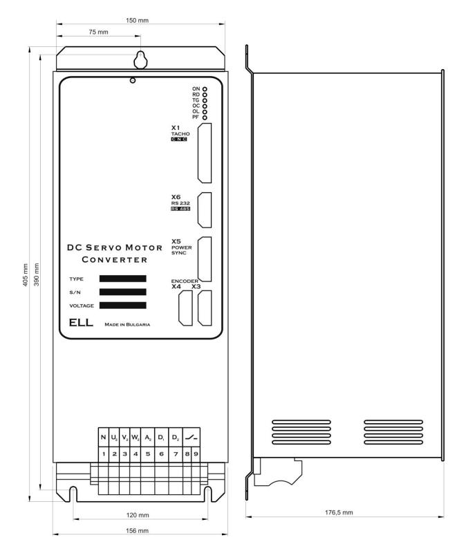
Figure 2 Connecting and overall dimensions of converters type 12060/250 WSM
