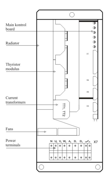
Figure 4 Positions of elements of converter type 12060/250 WSM
