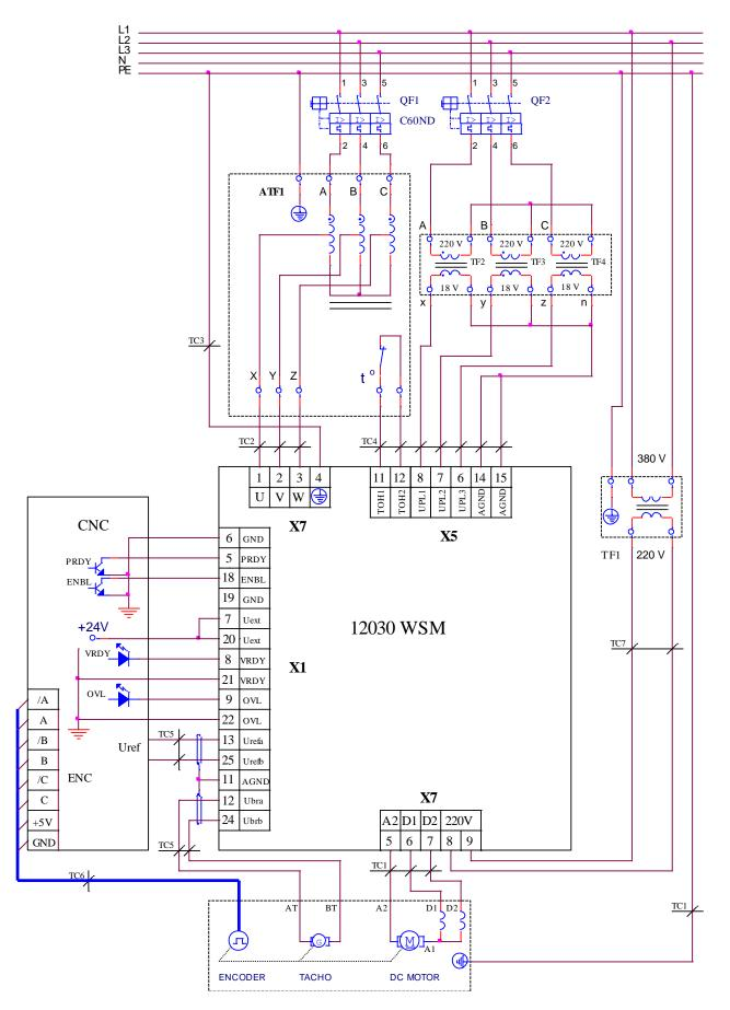
Figure 15 Connecting converters 12030 WSM to power supply autotransformer and separate group mono-phase transformers for operative supply and synchronization
