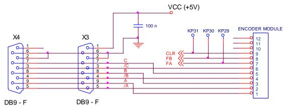
Figure 8 Electrical circuit and place of interface X3 pins for encoder and its extension X4
