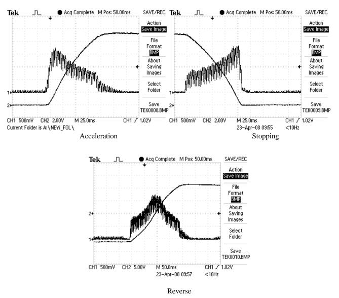
Figure 24 Speed and current curves when speed regulator is optimal adjusting
