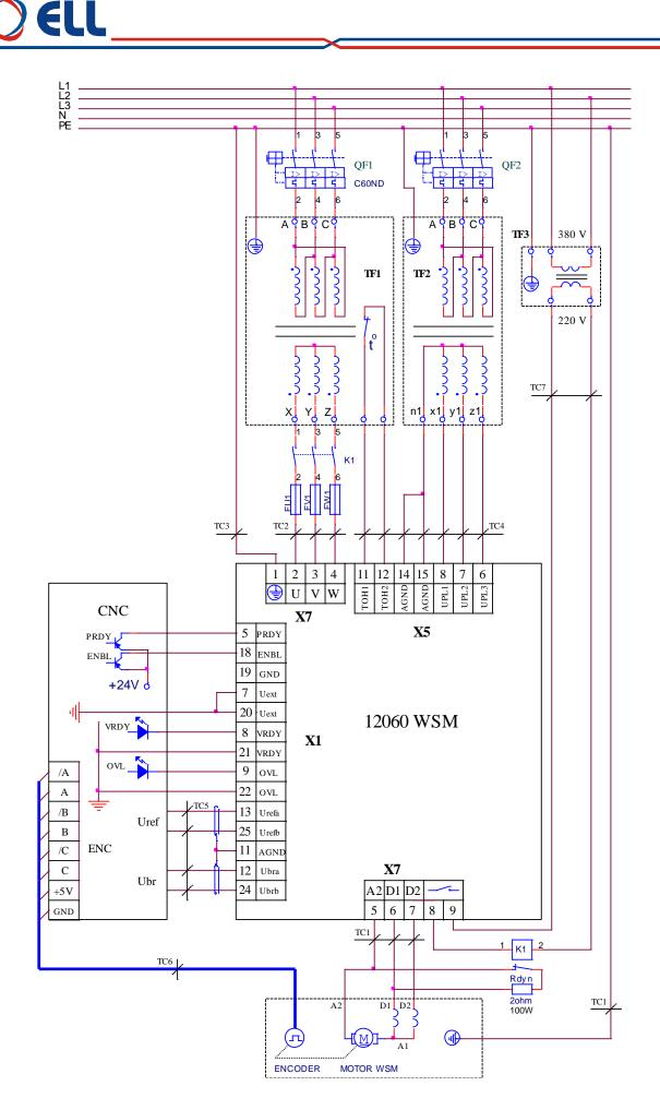
Figure 17 Connection the converter 12060 WSM to additional three-phase transformer with common three-phase operative and synchronizing coil
