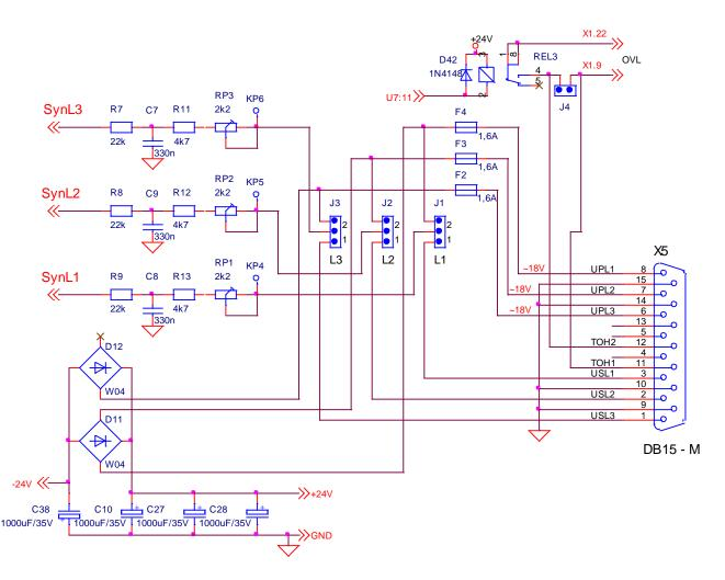
Figure 9 Principle scheme and pins of interface X5 for synchronizing and operative supply of converter control
