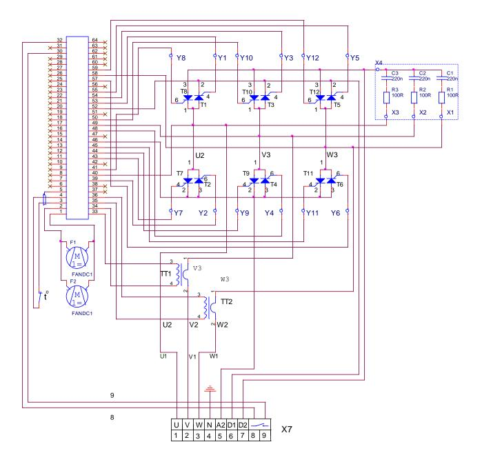
Figure 12 Electrical circuit of power block for converter type 12060 WSM
