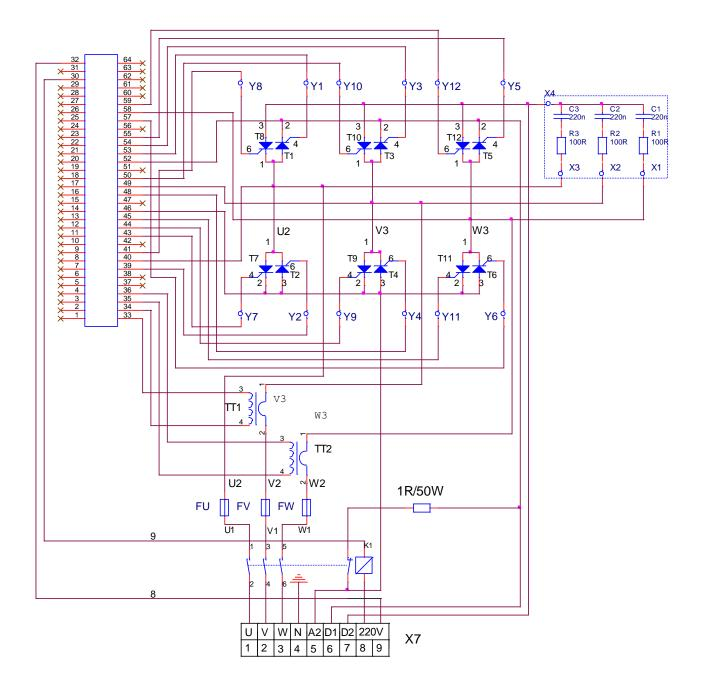
Figure 11 Electrical circuit of power block for converter type 12030 WSM
