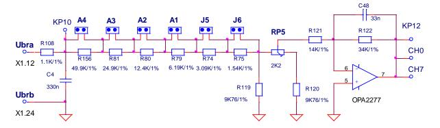
Figure 7 Structure of analog input for tachogenerator Ubr
