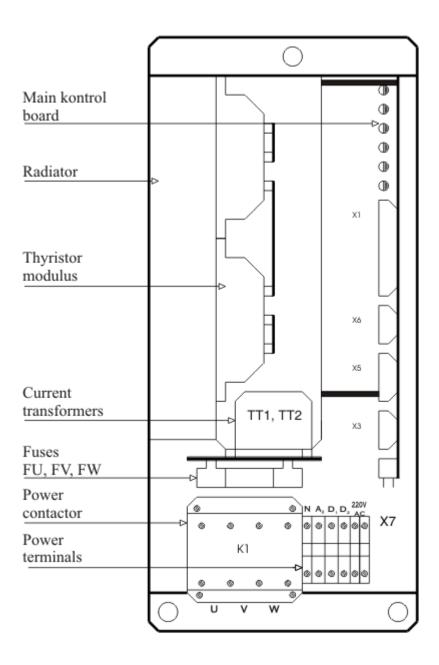
Figure 3 Converter type 12030/250 WSM elements positions
