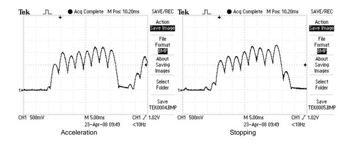
Figure 22 Current curves with over-regulating when parameter P06.01 has high value and parameter P06.02 has low value
