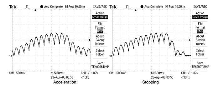
Figure 23 Current curve with lasting transient process when parameter P06.01 has low value and parameter P06.02 has high value
