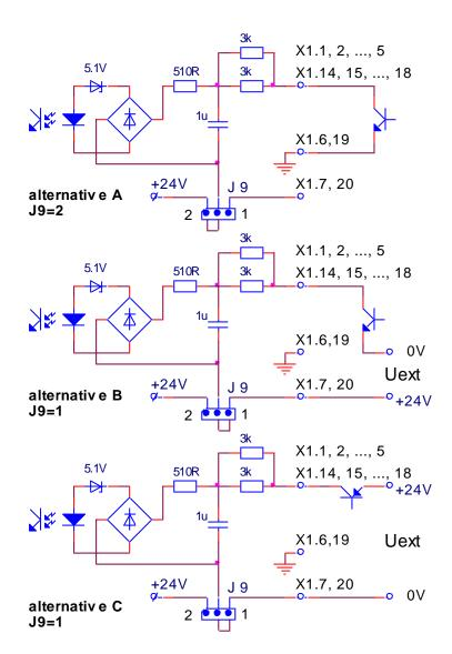
Figure 6 Structure of digital inputs
