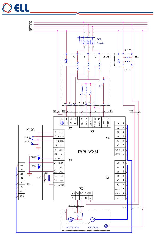
Figure 18 Connection converter 12030 WSM to power supply autotransformer with common coil for operative supply and synchronizing
