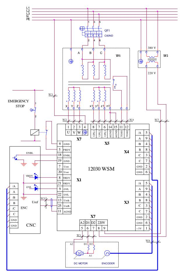
Figure 16 Connection the converter 12030 WSM to the mains transformer with common three-phase operative and synchronizing coil
